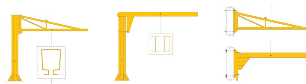
Gru a bandiera a colonna e mensola in rotazione manuale / Column-mounted and bracket mounted jib cranes with manual rotation
